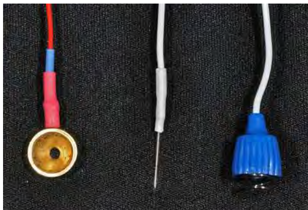
Fig. 1 Three examples of electrodes that can be used as ground and reference electrodes in the dog. The electrode to the left is a button-type cutaneous electrode. The cup is filled with a sticky contact paste, which makes contact with the skin and keeps the electrode in position. The electrodes in the middle and to the right both have needles that are inserted subcutaneously (middle: straight metal needle; right: cork screw-shaped stainless steel needle)
